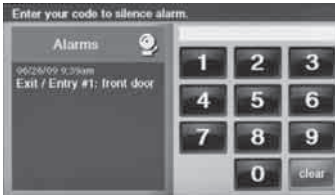
Disarm Screen Showing Alarms
