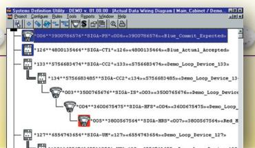
Signature Series input/output modules are powerful yet flexible devices that allow the life safety system to interact with the world beyond its Signature loop controller. The function of each module is determined by an installerselected personality code, which is set during system configuration. This exclusive Signature Series innovation provides elegant system interoperability at a fraction of the cost and time when compared with other methods.
