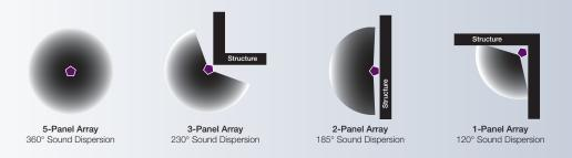
HS Series loudspeakers are available in a number of different configurations, from one panel configurations that provide a relatively narrow sound dispersion, to five-panel configurations with full 360° sound projection.
